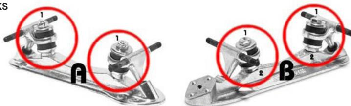
The stiffness of the trucks can also be regulated by replacing the cushions with harder/softer ones. Make sure during replacement that the cushions are the correct size and respect the manufacturer's recommendations.
